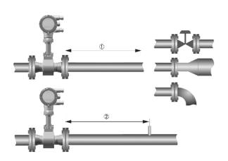
① Upstream of pipe expanders, pipe bends, control valves,
