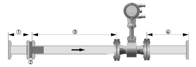
If, due to the type of installation, the required inlet sections are not available, the manufacturer recommends using flow straighteners. Flow straighteners are installed between two flanges upstream of the device and shorten the required inlet section.
