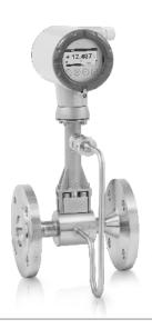
The FLOWIRL™ 8400 F1R / F2R with integrated nominal diameter reduction up to two nominal diameter sizes assures best results in accuracy and optimal measuring ranges even in pipelines with large diameters, designed for low pressure loss.
